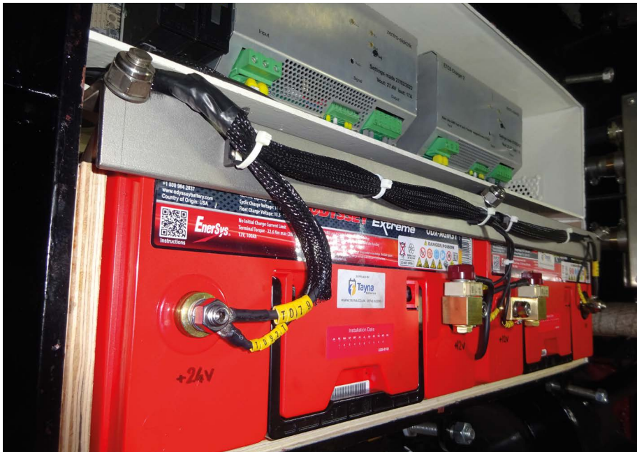
ETCS batteries fully connected with cable management in place.
