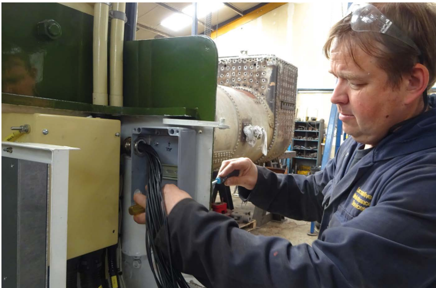
Andy Meredith attaching the new AS wiring box to the fireman's seat rear panel.
