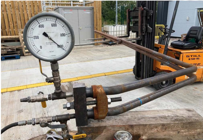
Above left: The rig used to test the superheater elements.
