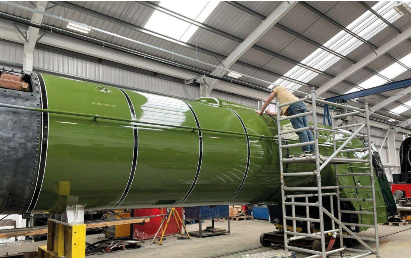
With the boiler painted, Ian Matthews starts to apply lining to the boiler bands. TCC
