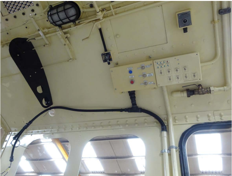
Fireman's side roof panel in place and wired with AWS/TPWS panel to the left of it.
