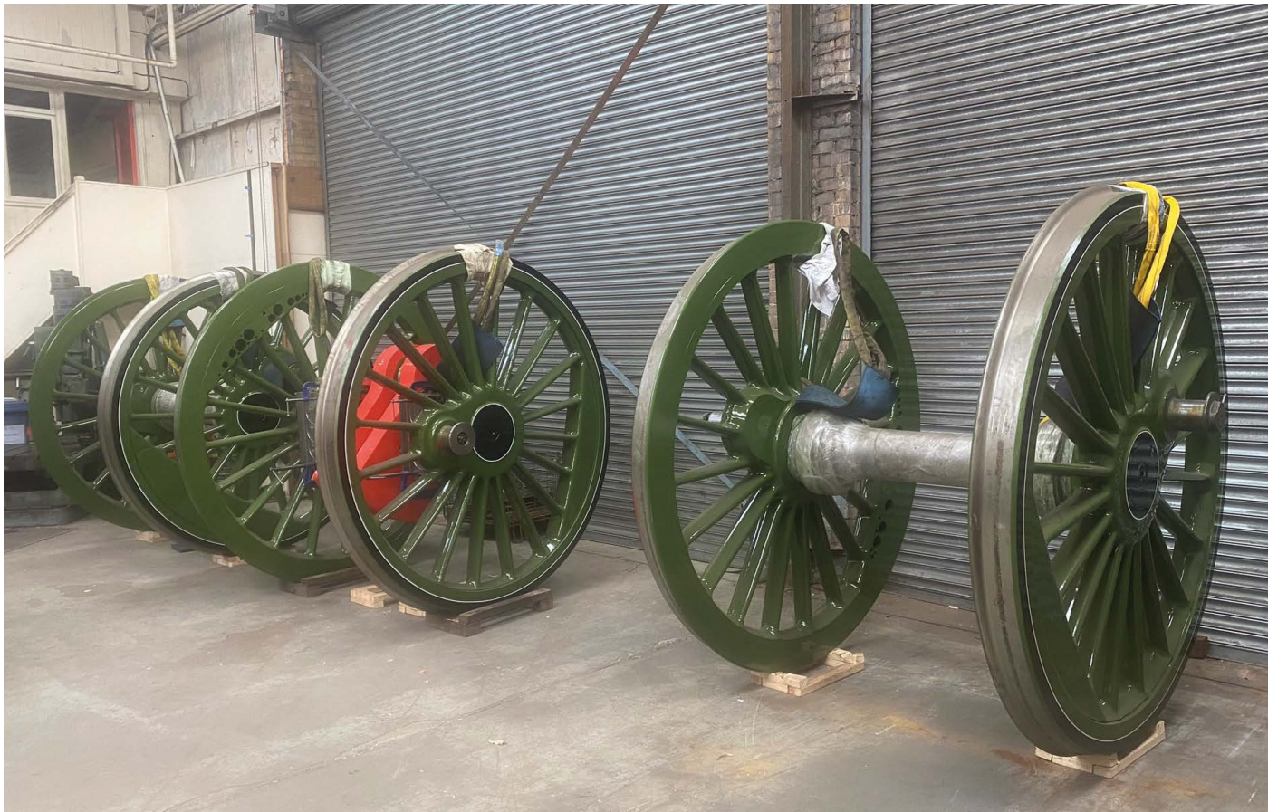
The three driving wheelsets fully painted and lined.
