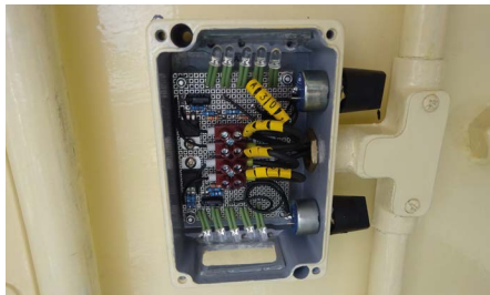
New LED light box to illuminate driver's and fireman's side roof panels.
