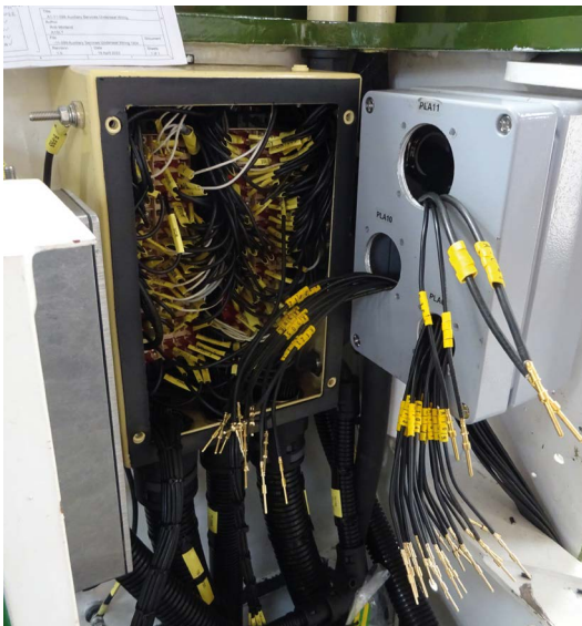
Andy Meredith attaching the new AS wiring box to the fireman's seat rear panel.
