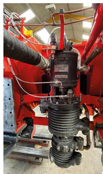
Above: The frames from rear showing rear air pump in place with insulated steam pipes being refitted.
