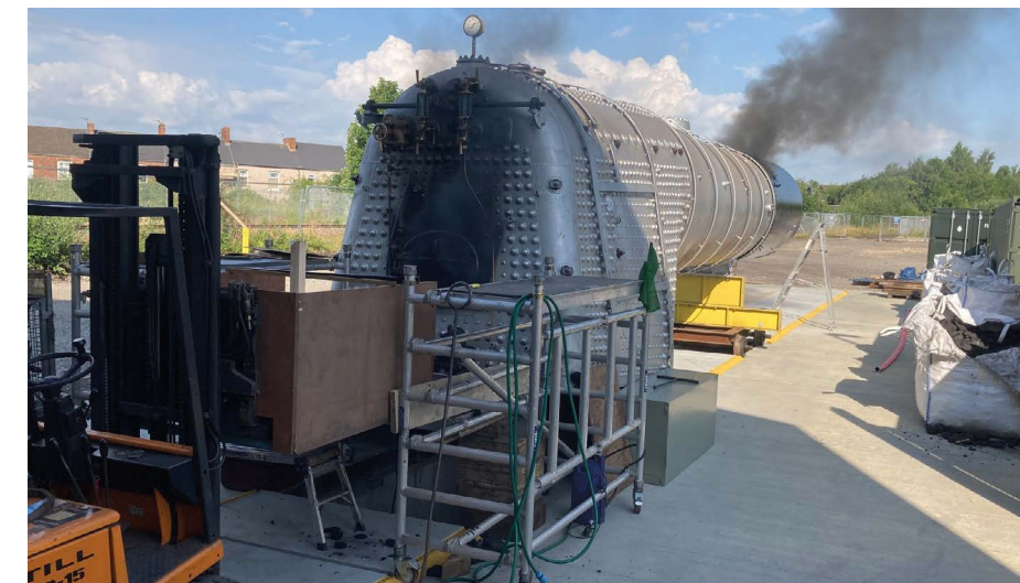
Right: The boiler set up for the steam test.
