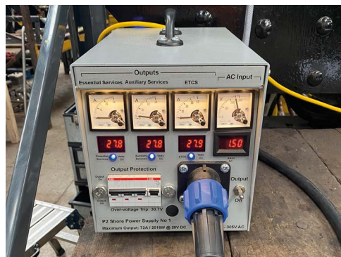
The external power supply unit designed and built by Rob in use supporting electrical testing.
