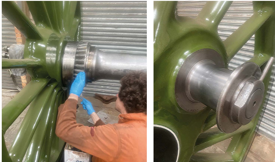
Alex Morton cleans the old grease from the left-hand roller bearing on the trailing wheelset.
