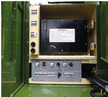
Above: ETCS I/O Panel in place on the front of the tender.
