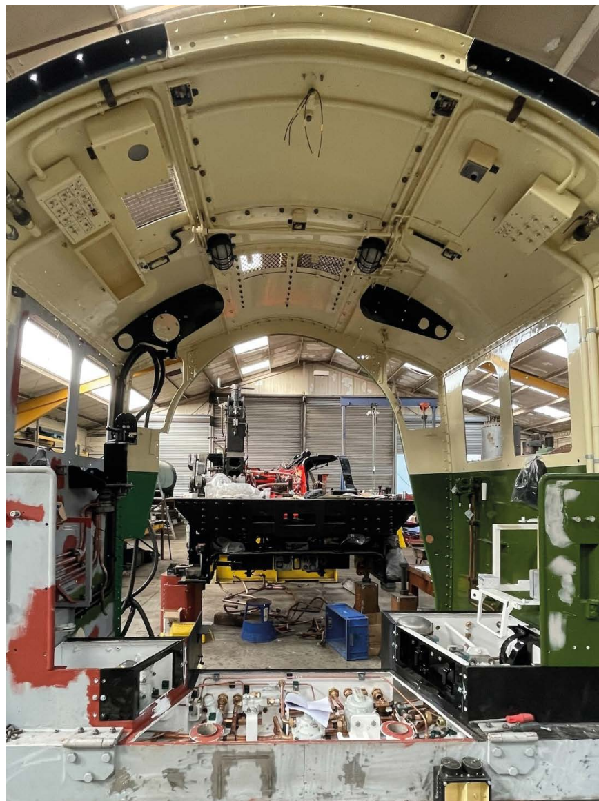
A view of the cab showing progress fitting new electrical boxes.
