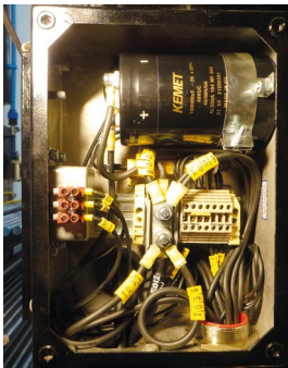
Above centre: Inside ADA connection box with wiring and over-voltage crowbar in place on the left.
