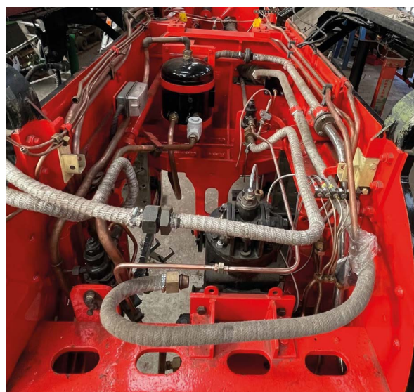
Above: The frames from rear showing rear air pump in place with insulated steam pipes being refitted.
