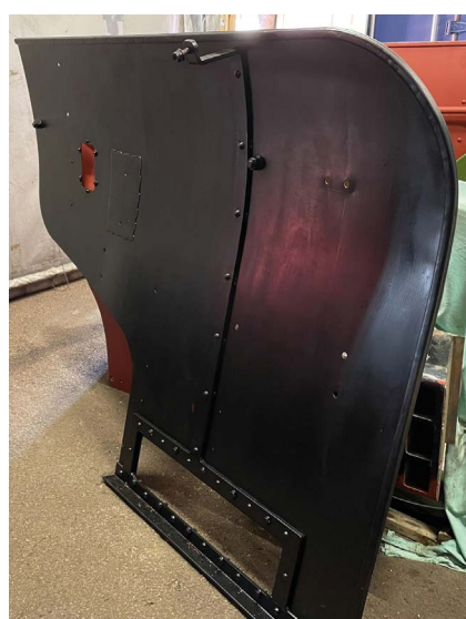
The driver's side smoke deflector with enlarged removable panel for access to the new ETCS turbogen.
