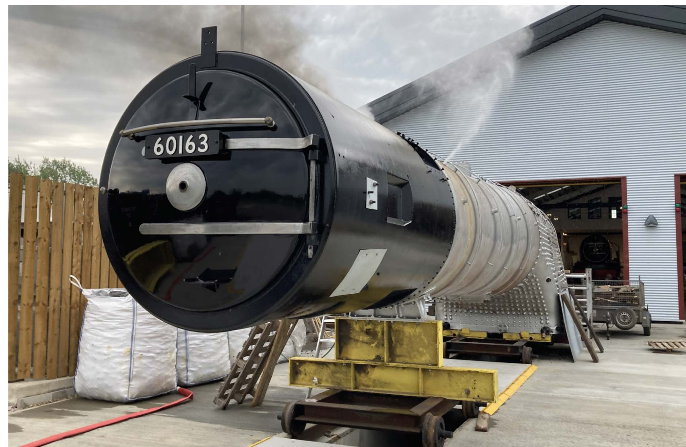
Steam starts to emanate from the boiler, issuing from open wash-out plugs at the front.
