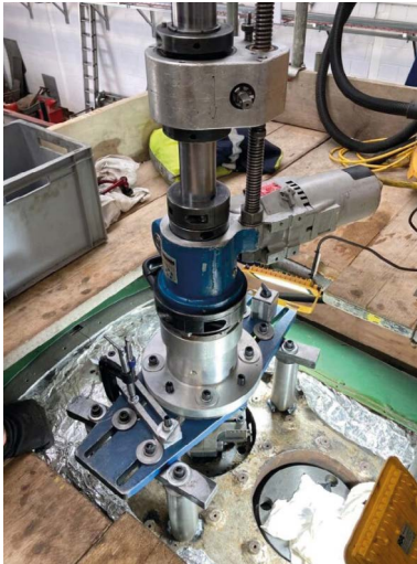
Above left: The rig used to test the superheater elements.
